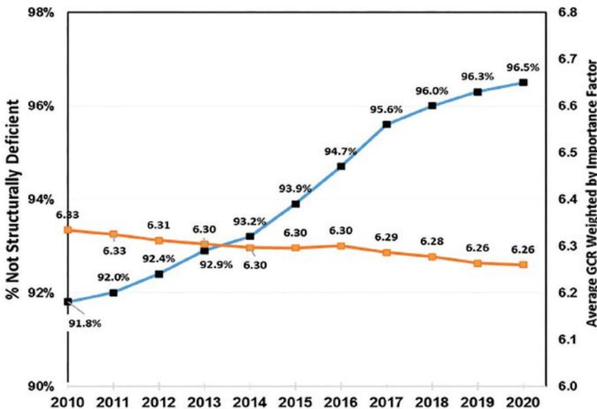
Figure 1. Percentage of bridges not structurally deficient (blue line) and average general condition rating (GCR; orange line) weighted by importance factor since 2010. All Photos and Figures: Virginia Department of Transportation.
