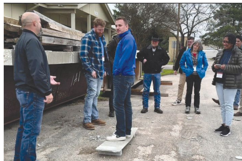
Figure 2. A course participant "walks the plank" in a demonstration of the strength and ductility of ultra-high-performance concrete.
