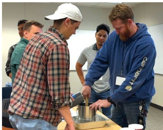
Figure 1. Participants in the Concrete Materials for Bridges course mix premeasured amounts of cementitious materials and water in a hands-on demonstration showing heat of hydration.
