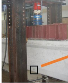
Figure 5. Cracking in a pretensioned concrete I-beam. 2
