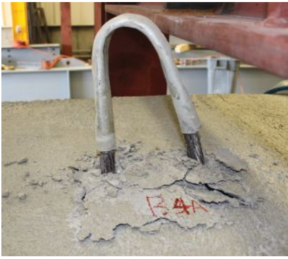
Figure 3. Researchers observed that failure modes varied depending on the configuration of the lifting loops. From left to right, the photos show pullout, strand rupture, and side-face blowout failure modes. Photos: University of Cincinnati.
