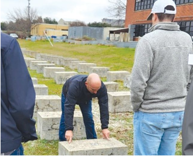
Figure 3. During a tour of concrete exposure sites, Dr. Thano Drimalas describes expansion measurements on specimens.
