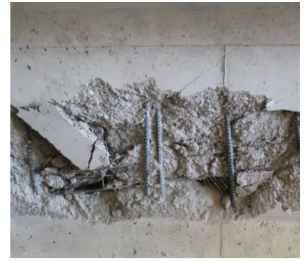
Figure 3. Researchers observed that failure modes varied depending on the configuration of the lifting loops. From left to right, the photos show pullout, strand rupture, and side-face blowout failure modes. Photos: University of Cincinnati.
