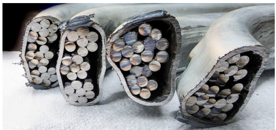
Figure 2. Comparison of multiple-strand loops with crushed and uncrushed pipe sleeves. Uncrushed pipe sleeves do not adequately keep the individual strands together and at the same elevation. Photo: Prestress Services Inc.
