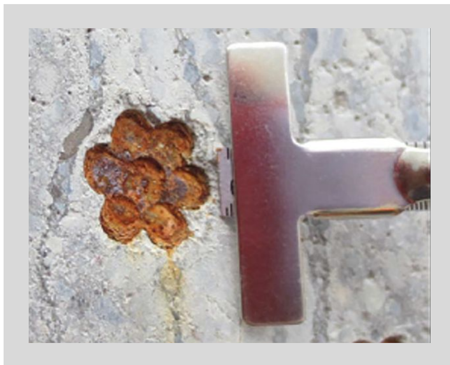
Figure 3. An example of a strand draw-in measuring device. 1
