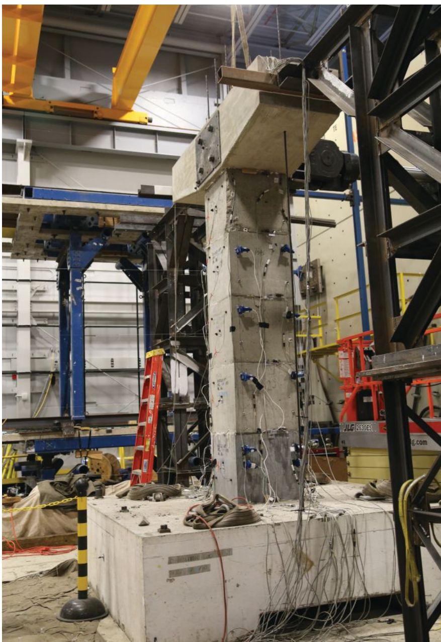
Testing of a precast concrete rocking column with ultra-high-performance concrete at the base column segment. Photo: Dr. Cancan Yang.
