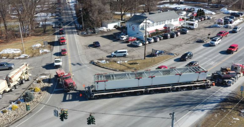
A precast concrete U-beam segment is transported to the dock facility in Albany, N.Y., before being shipped by barge to the project site. Photo: Fort Miller Precast.
