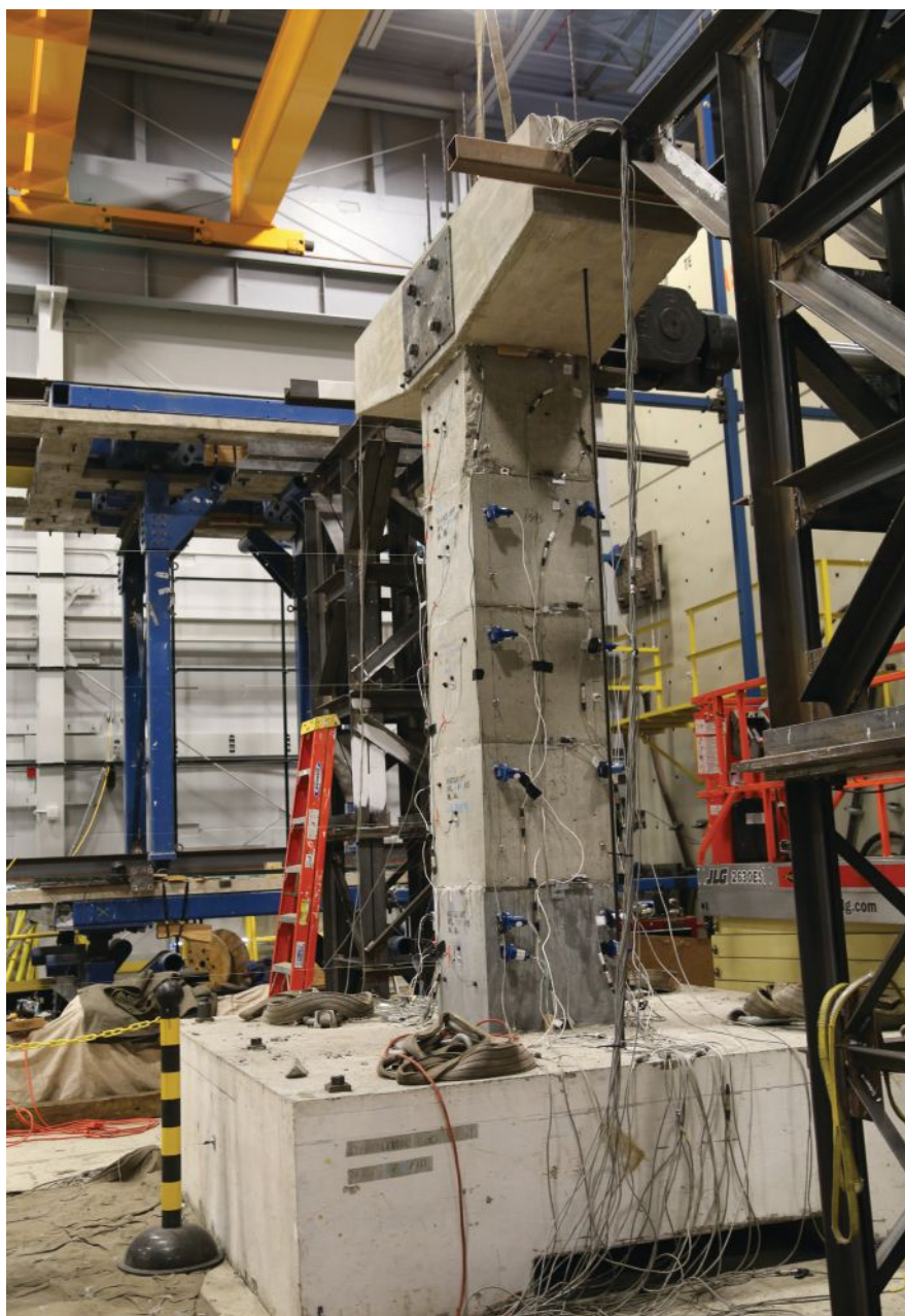
Testing of a precast concrete rocking column with ultra-high-performance concrete at the base column segment. Photo: Dr. Cancan Yang.
