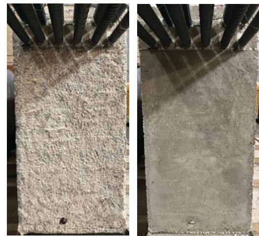
Figure 3. Different levels of interface roughness: intentionally roughened interface on the left and form-finished interface on the right. 1
