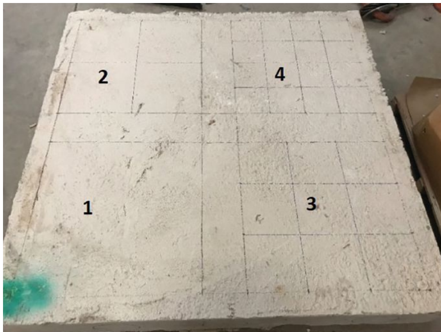
Figure 1. Saw-cutting patterns on the slab specimens help establish the relationship between time and air-pollutant emissions during partial-depth concrete deck repair methods. All Figures: Courtesy of Israi Abu Shanab.
