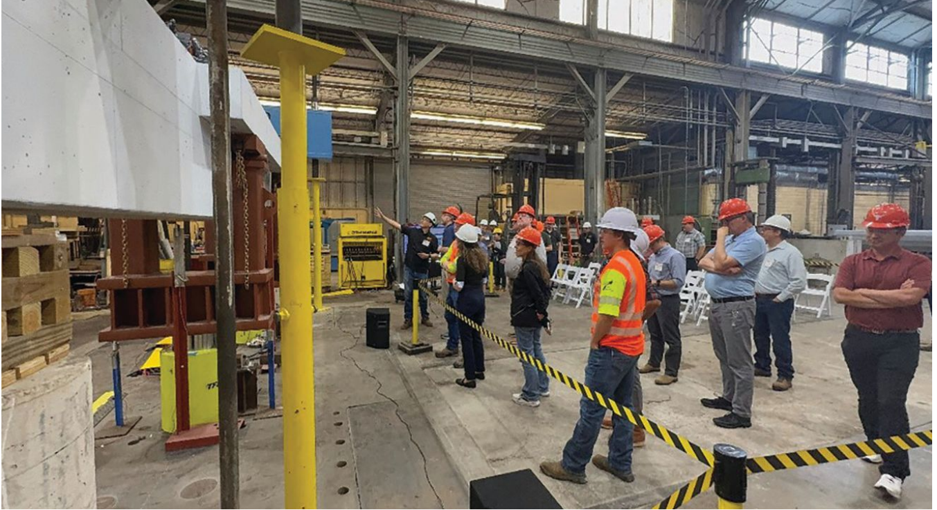
Structural behavior predictions for an inverted tee specimen are tested at the CBEI Conference and Workshop.
